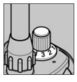
1) Turn the selection dial of handheld transmitter to the desired number to pair it with the receiver. (For example, if you want to designate a receiver as your number 2 receiver, set the selection dial of the transmitter to number 2.)
