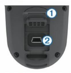
2 Plug the small end of the power cable into the mini-USB port ② on the device.
