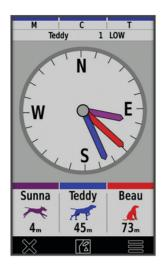
You can use the dog tracking compass to view the direction and distance to your dog, your vehicle, and any paired devices. The dog tracking compass also shows the dog's status, such as running or on point (*Dog Status Icons*, page 13). The color of the pointer corresponds to the color of the track.
