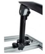
5) Slide the base of the launcher tube into the circular clamp. Drop the tube onto the post of the mounting plate. Once the tube is pushed completely down and securely in position slide the circular clamp down to the mounting plate.
