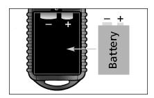
The larger battery terminal should touch the larger transmitter contact.
