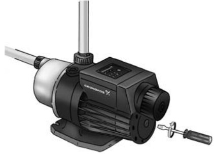
Fig. 17 Removing the end-cover plug
