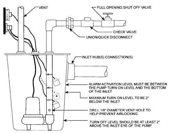
\* CONTROL CAN CONSIST OF ONE FLOAT, OFTEN WITH SERIES (PIGGYBACK) PLUG OR WIRING, OR TWO FLOATS OPERATING A RELAY.
