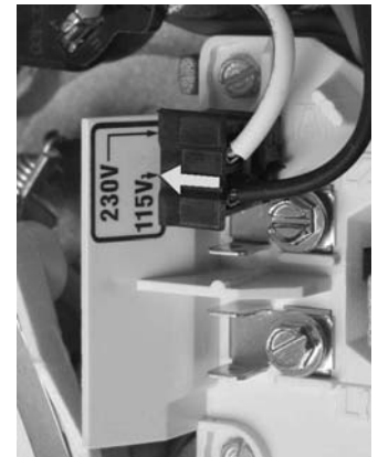
Figure 4B Voltage Change Plug Set for 115 Volts
