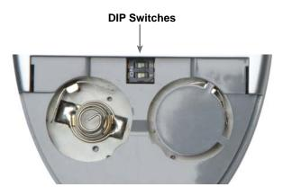
It is important that the IR channel selected on the remote, match the IR channel on the GefenToolBox 4x1 Switcher for HDMI for proper operation. For example, if you set both DIP switches on the remote to the down position (toward the "1" and "2"), IR channel 0, you must set the GefenToolBox 4x1 Switcher for HDMI to use IR channel 0.
