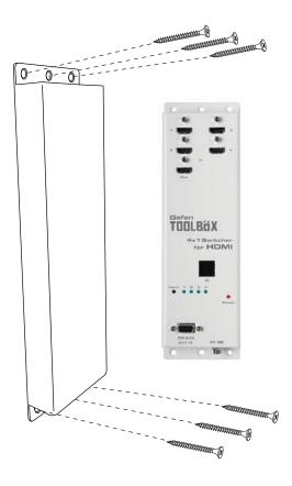
The GefenToolBox 4x1 Switcher for HDMI should be mounted vertically in a wall or cabinet with wood/drywall screws as shown in the diagram above. There should be an inch or two of clearance between the edges of the unit and any walls or vertical surfaces to allow for enough clearance for insertion and retraction of cables at the HDMI connectors.
