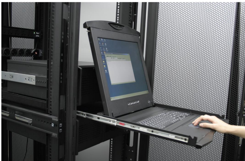
Figure 6. Operating the LCD keyboard drawer
