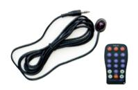
**IR**: Many system proffesionals prefer the IR control interface because it offers greater flexibility to manage the CATSwitchPro at a distance. In some cases, the displays will not be visible from the matrix. In these situations it is necessary to control the matrix with Infrared control.
