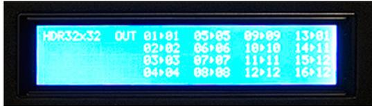
The MXCore-UD front panel enables one to switch directly from the Matrix without the use of any software.
