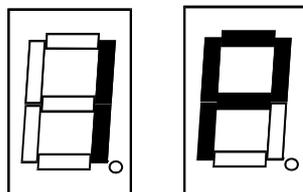
SmartView has powered up normally and there is sufficient power available from the connected PCs
