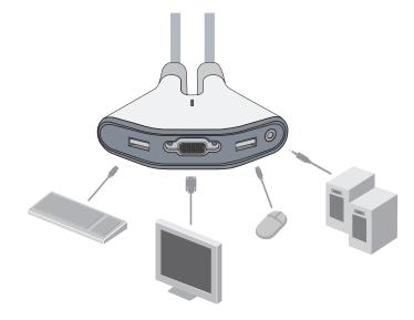
3. Connect one set of cables to the monitor, USB, and speaker ports on your first computer. Wait for your computer to recognize the new USB device (Flip). Then connect the other set of cables to the monitor, USB, and speaker ports on your second computer. If the cable is not long enough to connect to your speaker port, use the included audio extension cable.
