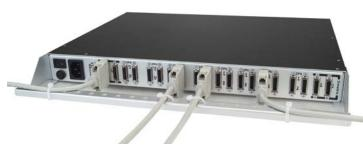
**High Density KVM Matrix Switch** with Cable Management Shelf (Standard feature for -UHD switches)
