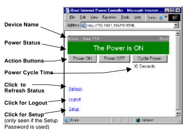
To control the power, click on the appropriate button. During power cycling, the Power Status bar will indicate the temporary status, with a blue background. Once the cycle is complete, the status bar will revert to its original condition. To abort a power
