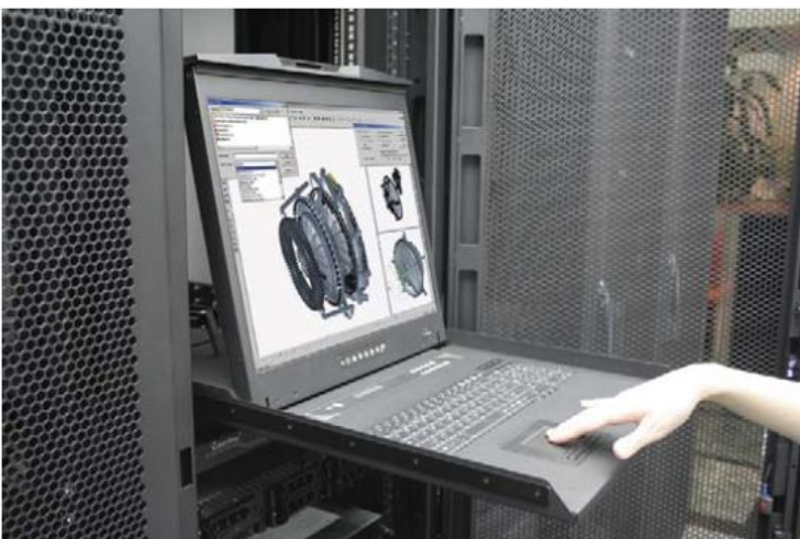
Figure 6. Operating the LCD keyboard drawer
