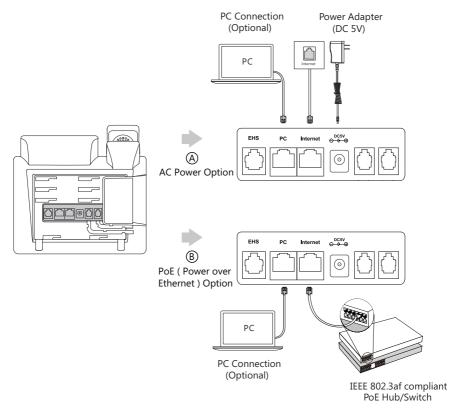
Note: The IP phone should be used with Yealink original power adapter (5V/1.2A) only. The use of the third-party power adapter may cause the damage to the phone. If you are connecting a PC to your phone, we recommend that you use the Ethernet cable provided by Yealink. If inline power (PoE) is provided, you don't need to connect the power adapter. Make sure the hub/switch is PoE-compliant.
