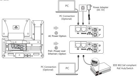
Note: The IP phone should be used with Yealink original power adapter (5V/2A) only. The use of the third-party power adapter may cause the damage to the phone. If you are connecting a PC to your phone, we recommend that you use the Ethernet cable provided by Yealink.
