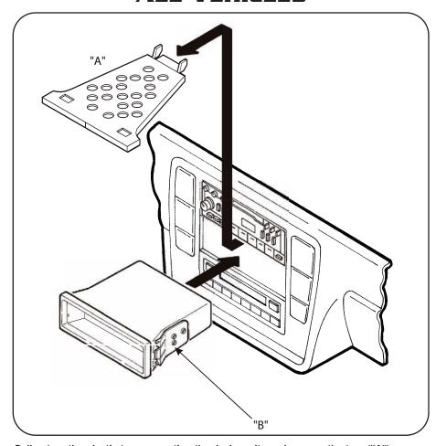
Pull out on the plastic tray separating the dash cavity and remove the tray ("A"). Position the Pocket so each Bracket is configured with (2) screws on the top and (1) screw on the bottom ("B"). Slide the Pocket into the dash opening until the side clips engage.
