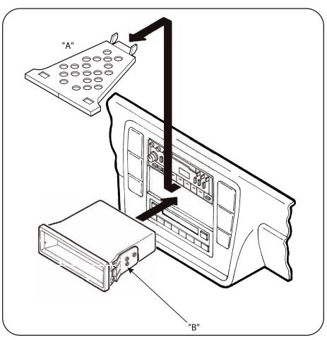
Pull out on the plastic tray separating the dash cavity and remove the tray ("A"). Position the Pocket so each Bracket is configured with (2) screws on the top and (1) screw on the bottom ("B"). Slide the Pocket into the dash opening until the side clips engage.
