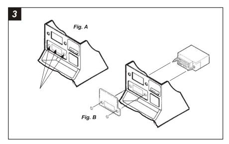
Using a dremel tool, cut the plastic along the scribed lines ("A") until the shaft holes and nose hole is formed. (see Fig. A). Slide the aftermarket head unit through the holes in the console and kit and secure with shaft nuts. (see Fig. B)
