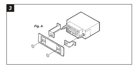
**2-SHAFT HEAD UNITS:** Slide the aftermarket head unit through the Faceplate and **Mounting Brackets** and secure with shaft nuts. (see Fig. A). Skip to the Installation Instructions for ALL VEHICLES on Page #5.
