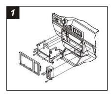
Disconnect the negative battery terminal to prevent an accidental short circuit. Unclip the radio trim bezel and remove. Remove (3) Phillips screws securing the trip computer and remove. Remove (7) Phillips screws securing the factory radio assembly and disconnect the wiring.
