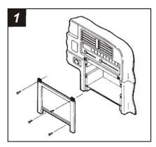
Disconnect the negative battery terminal to prevent an accidental short circuit. Remove the cupholder and (2) screws exposed. Remove the ashtray and (2) screws exposed on the ashtray bracket. Unclip the radio trim bezel and remove. Remove the screws securing the factory head unit and disconnect the wiring.
