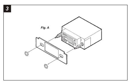
**2-SHAFT HEAD UNITS:** Slide the aftermarket head unit into the kit and secure with shaft nuts. (see Fig. A). Skip to the Installation Instructions for ALL VEHICLES on Page #5.
