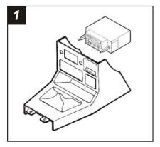
Disconnect the negative battery terminal to prevent an accidental short circuit. Remove (4) screws securing the dash console, lift the console out and disconnect the wiring.
