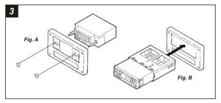
**2-SHAFT HEAD UNITS:** Slide the aftermarket head unit into the kit and secure with shaft nuts. (see Fig. A). Skip to the Installation Instructions for ALL VEHICLES on Page #5.
