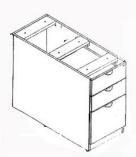
Step 1: Assemble false pedestal using cam locks and pins provided. Then attach drawer pulls and leveling glides to pedestal.
