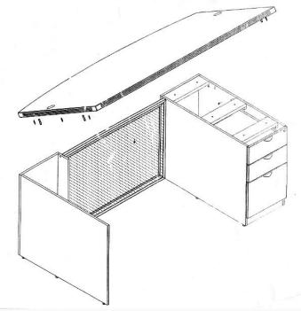
Step 4: Attach file pedestal(s) to desktop using the 6 bolts provided.
