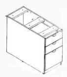
Step 1: Attach leveling glides and drawer pulls to pedestals
