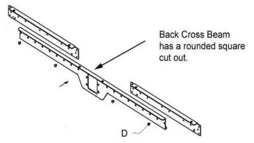
4.) Attach the back cross beam to the adjustable leg frame using two (D) screws per side.
