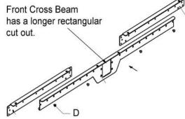
9.) Place Front Cross Beam so that the motor fits through the cutout. Attach motor with two (D) screws. Then, attach the front cross beam to the adjustable leg frame using two (D) screws per side, like shown in Step 4.
