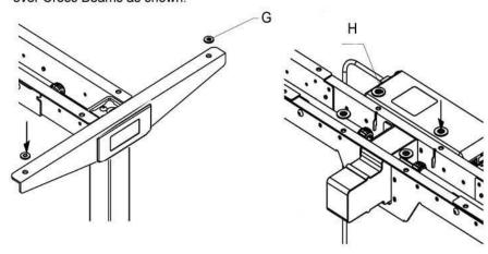
15.) It is time to mount the desktop. With a helper, lay the desktop on top of the assembled frame, making sure the front and back edges are flush with the desktop brackets and that there is 2" of desktop overhang on the side panels.
