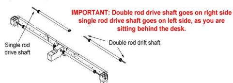
The Drive Shafts twist open and closed. Twist both open to allow you to slide the metal rod in and out of the shaft. Twist both shafts open and insert into motor and adjustable leg frames.
