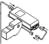
12.) Plug the power cord into a power outlet. Using the handset, raise the adjustable legs a few inches to make attaching the Desktop Brackets easier. Attach the Desktop Brackets with two (E) M6x8 Screws each.
