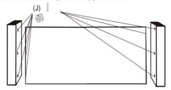
3.) Now, assemble the Back Cross Beam with two Cross Beam Supports, using the (D) M8x20 Machine Screws. Use two D screws to attach each Cross Beam support. Make sure length of entire cross beam matches the width of the desk.
