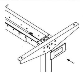
14.) Place (G) Washers on the Desktop Brackets as shown. Place (H) washers over Cross Beams as shown.
