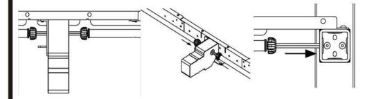
7.) Use (C) Wrench to tighten Drive Shafts.
