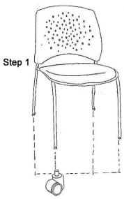
Step 1: Snap four (F) Casters into (E) Steel Frame by hand
