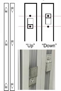
Step 3) Slide your second panel into your first panel by slightly tipping the second panel and dropping the brackets down into the first panel. Brackets will fit together. Repeat Steps 1 & 2 as needed.
