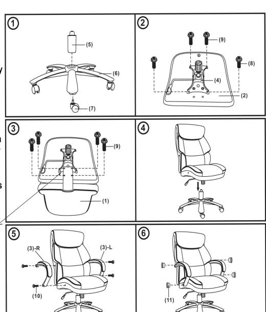
Screws are located in the holes. Use Allen Wrench to back them out for assembly.
