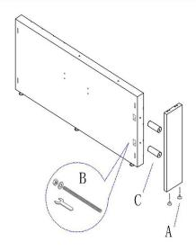
1.) Install (A) Leveling Glides in ALL Panels. Then, attach Front Panel to Side Accent Panel by threading the (B) Bolt/Washer/Nut hardware through the (C) Accents Posts. Use the Wrench included to tighten bolts in the two cut out areas.
