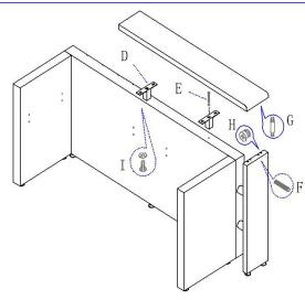
3.) Now, mount the (D) Counter Supports to the Front Panel using the (E) Screws/Washers. Then, attach the Counter Top to the Accent Panel using the (H) Cam Locks, (G) Cam Pins and (F) Wood Dowels. Twist the (H) Cam Locks with a Phillips Screwdriver to tighten. Finally, use the (I) Screws/Washers to connect the Counter Top to the (D) Counter Supports.
