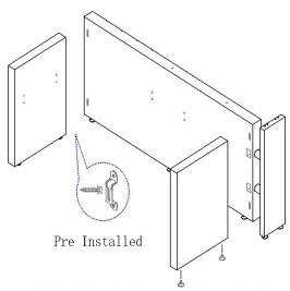
2.) Next, attach the Left & Right Side Panels to the Front Panel by inserting the heads of the screws (that insert into the Side Panels) into the pre-installed brackets.
