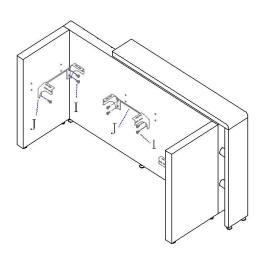
4.) Attach the (J) Desktop Support Brackets to the interior area of the desk as shown above. Use the (I) Screws/Washers.
