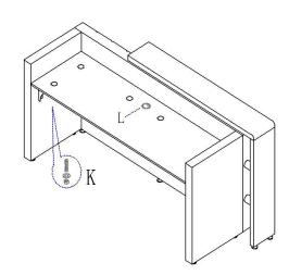
5.) Attach the Desktop to the (J) Desktop Support Brackets using the (K) Screw/Washer/Nut hardware. Then, your last step is to insert the (L) Grommet into the Desktop.
