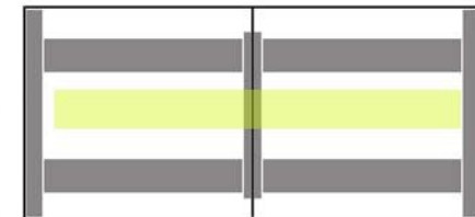
Positioning of Shared Cable Troughs shown in yellow
