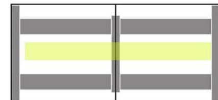
Positioning of Shared Cable Troughs shown in yellow
