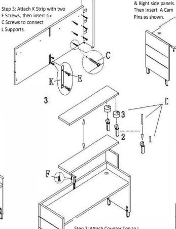
Step 7: Attach Counter Top to I Counter Support using two F Screws as shown. Then, attach D hardware assembly into the vertical support for the counter.
