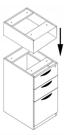
Step 2.) Unpack your Open Storage Cubby from its box. This unit attaches to the top of file pedestal using 4 bolts.
