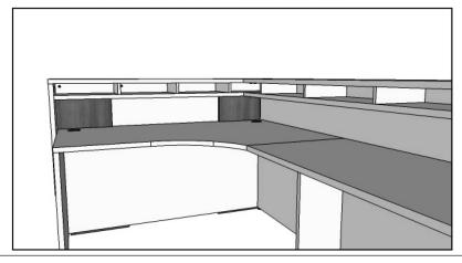
Insert the connector bolts and tight clockwise securely.
