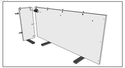
Then position the other back and shelves (pre-assembled) in line with the first back. Align the pins and holes slide into position and tighten the 3 connectors clockwise.
