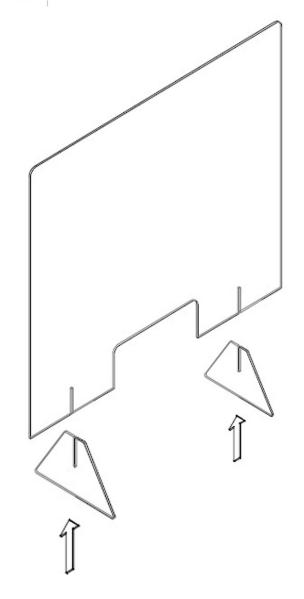
Step 1.) Insert Wedge Feet into Shield by hand.
