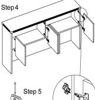
4.) Your next step is to attach the hutch doors. See Figure "B" which identifies the Outside Doors and Inside Doors. There are different hinges that connect the inside & outside hinges.
