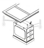
Step 5 Install flat bracket, centered over seam between executive desk and return desk, on the UNDERSIDE of the desk surfaces. Use the wood screws provided.
