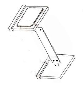
3.) Next, put the metal pins into the holes of the bases and place the cam locks into the pre-drilled holes of the support beam. Line up the holes of support beam to the bases so that the pins go into the support beam holes. Once in place, tighten the cams with a Phillips screwdriver by turning until locked and secured into place.
