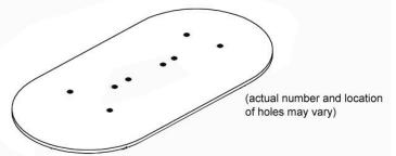
3.) Attach your first base. First, insert any cam locks in the base. Align the holes at the top of the base over the cam pins and dowels. Set base down over holes. To secure, twist cam lock with a Phillips Screwdriver like shown in the diagram.
