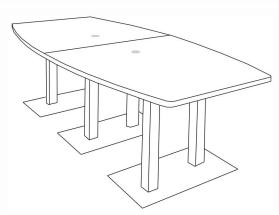
Step 1) Assembling The Bases. Start by attaching the A Plates to the B Columns. Then, turn that assembly upside down to attach the C bases. This will help align the holes easier. Finally, once the bases are fully assembled, carefully turn them over so that C bases are on the ground.
