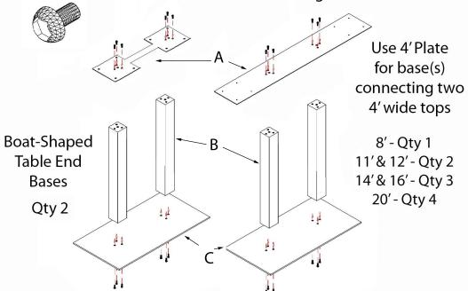
Step 2: Arrange Assembled Bases. With a helper, set the tops on the bases to line up the holes on the tops to the bases.
