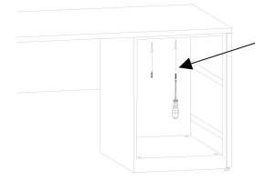
**Step 3**: Remove upper drawers as necessary and install supplied #8 x 1½" pan head screws (holes are pre drilled in pedestal top) to secure pedestal to desk.
