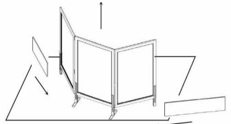
Step 4: Optional: If you plan to raise the shields, loosen the screws of the Add-on Clamps and slide the Acrylic Side Screens In. This will be a tight fit so the screen will stay positioned and may require a rubber mallet to gently tap in.
