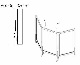
Step 2: If you purchased your shield with add-on wings, slide the hinge(s) of the add-on(s) into the hinges of the center shield.
