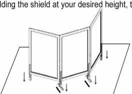
Step 3: For stability, secure the feet of the Center Shield by either applying the double sided adhesive tape (included) to the feet or by drilling the self-drilling screws through the holes of the feet into your surface.
