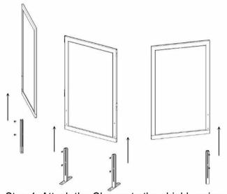
Step 1: Attach the Clamps to the shields using the M6\*8 screws and Allen Wrench provided. To adjust the height of the shields, leave the screws loose and with a helper holding the shield at your desired height, tighten down.
