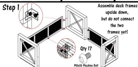
Step 1) Determine if you want a Left or Right Return. A Left Return is shown above. Assemble the main desk and return desk frames independently, using a screwdriver.
