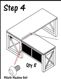
Step 4) With a helper, turn both desk sections over, right side up. Then, attach the return desk to the main desk using two M6x16 Bolts. Also, attach the Flat Bracket over the seam of the two desk sections using six M6x16 Bolts.
