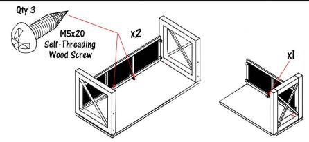
Step 3). Using the M5x20 Self-Threading Wood Screws and a Power Screwdriver, attach the modesty panels to their respective worksurfaces. The screws are self-threading, so you will make your own holes.
