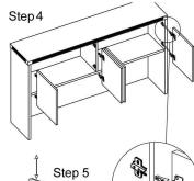
4.) Your next step is to attach the hutch doors. See Figure "B" which identifies the Outside Doors and Inside Doors. There are different hinges that connect the inside & outside hinges.
