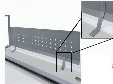
Step 1: Modesty Panel is easiest to attach when desk is upside down. Attach the two angled brackets to the modesy panel itself with the four bolts and washers provided. Screw silver caps on other side of panel once done.
