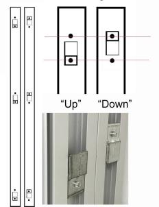
Step 3) Slide your second panel into your first panel by slightly tipping the second panel and dropping the brackets down into the first panel. Brackets will fit together. Repeat Steps 1 & 2 as needed.
