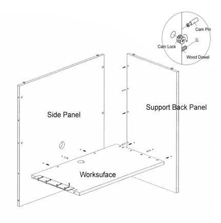
Picture shows a left return being assembled, upside down.
