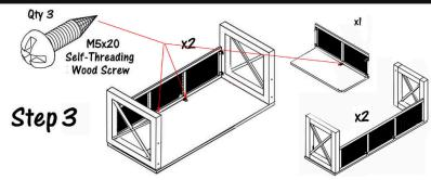
Step 3). Using the M5x20 Self-Threading Wood Screws and a Power Screwdriver, attach the modesty panels to their respective worksurfaces. The screws are self-threading, so you will make your own holes.
