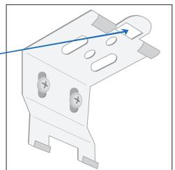
**Mount the headrail.** Position the headrail with the back panel **(A)** resting on both bottom hooks of all brackets. Push the front of the headrail firmly upwards and toward the wall until the groove at the top of the headrail snaps into place, **(B)** as shown.
