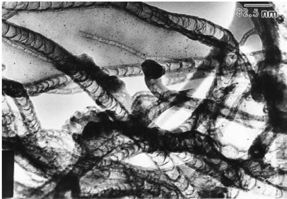
Figure 8. TEM of electrospun mixture of bamboo structured fCNTs in Estane/PANI-SPS(1M).
