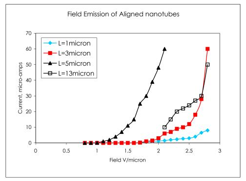
Fig 4. Short nanotube emitters have higher onset than longer ones, although the 13 micron emitter has a lower onset than the 5 micron set. All samples have 1cm2 area.
