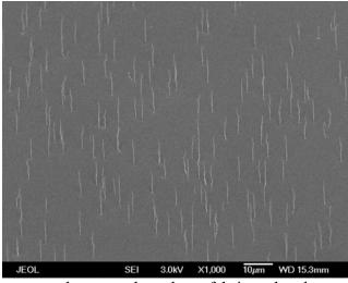
Fig. 7. Lower density nanotube arrays have been fabricated and are now being measured.
