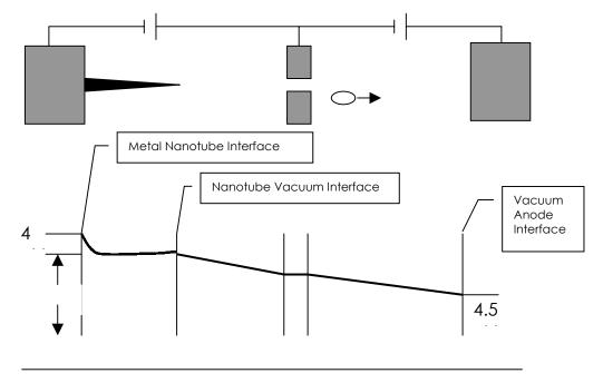
Figure 1. Under electric field, electrons tunnel from the material into vacuum.
