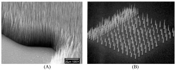
Figure 2A,B. Nanotube arrays grown by CVD can be uniquely tailored for various applications
