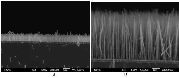
Fig. 3. Edge on views of nanotube arrays, show the variation of nanotube length.
