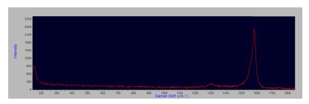
G:D band intensity ratio = 2340/240 = 9.75 Diameter = 233/155cm<sup>-1</sup> =1.5nm
